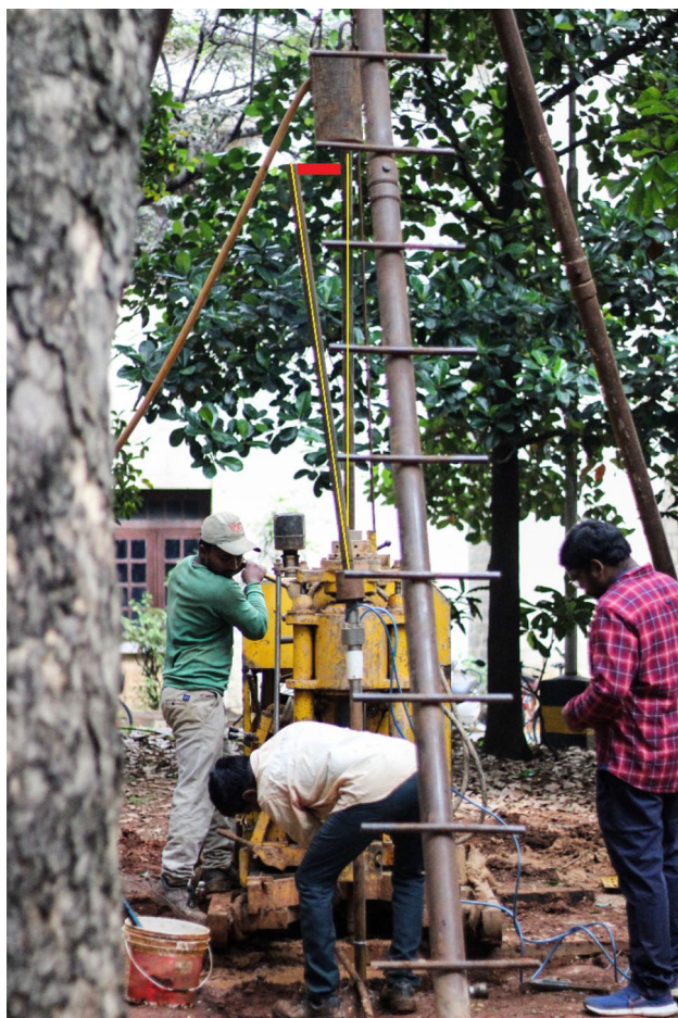
Fig. 4 Inclination of guide rod with respect to vertical rod fixed on drill rig
