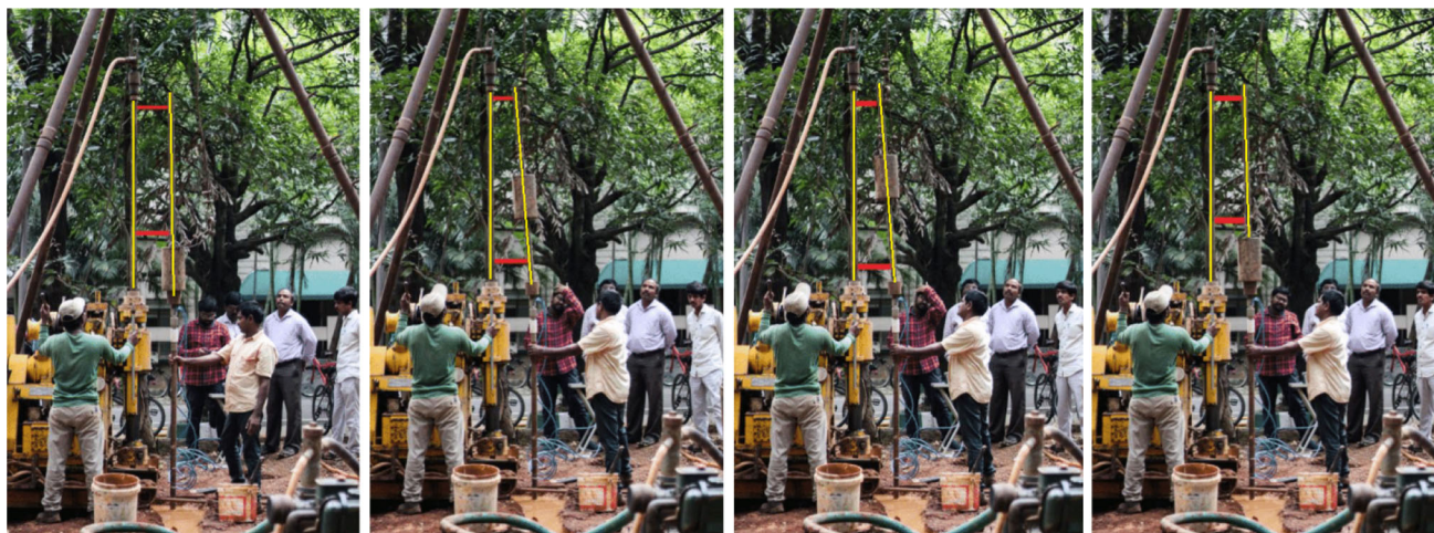
Fig. 5 Hammer lifting and releasing during a typical blow of HRL equipment showing inclination of guide rod during the operation of hammer lifting
